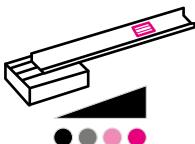
A charge indicator is built into the 11.4Ah and 19Ah batteries. Each of the 4 LEDs represents 25% of the total capacity. When the red LED starts flashing, there is approximately 10% of battery life remaining. The battery must be recharged after each day of use.
